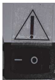
Figure 2-2. Battery Preserve Switch. See location at “The bkSpecto System” .
